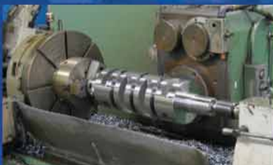
Ability to turn a raw billet into a crankshaft for any application up to 40" length and 10" diameter.
