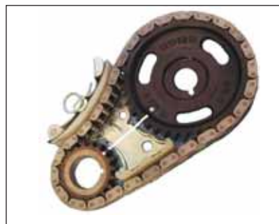
Figure 2 White line and dots mark correct timing for 1994-2003 GM 2.2L engines. Note cam dowel and crank keyway locations.
