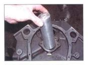
Photo 1 (above); Photo 2 (below) After the tool has been inserted into the block a .375" pilot is inserted into the tool,
