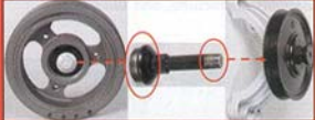
Figure 15 Front water pump applications have a crankshaft pulley, which is threaded for a stub shaft that is also threaded for the pulley belt drive assembly and mount. Both the stub shaft and belt drive pulley are left hand thread (red circles) and require a special long deep well socket to remove the stub shaft.
