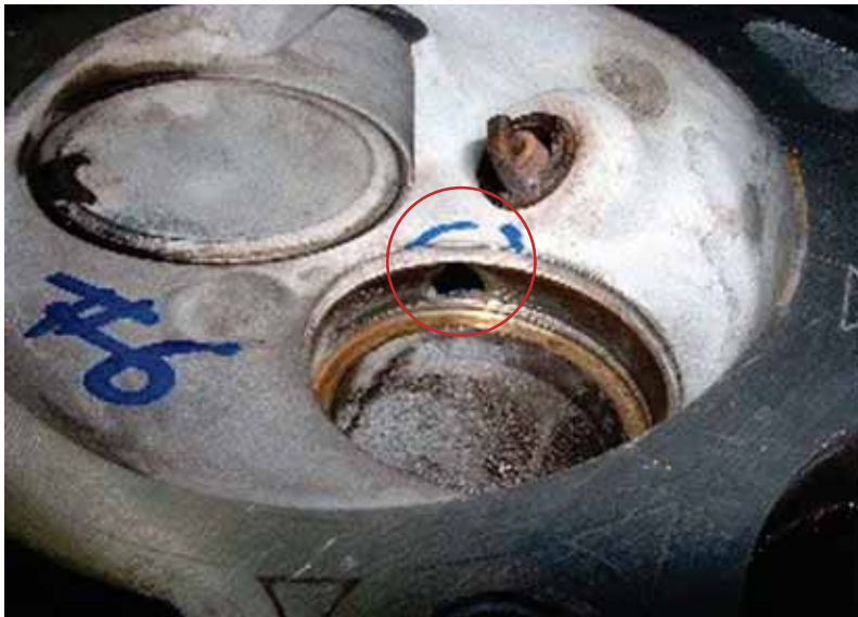
Figure 4 Hole exposed after removing valve seat on 1999-2003 Ford 5.4L engines.
