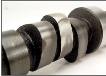
Figure 3 Use only the manufacturer-recommended lubricant, which is generally included with the cam.
