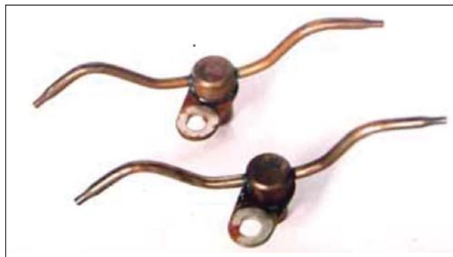
Figure 9 A whine sound may be present at idle after vehicles with 6.1L Hemi engines have been driven in warm ambient temperatures over 50° F (10° C). This sound can be caused by the piston oil cooler jets fluttering during hot oil/idle conditions.
