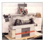
Winona Van Norman's VSG-4720 has enough spindle-to-table clearance to machine all the oldstyle blocks with valve seats including Ford 8N tractor engines and any other flathead engine.
