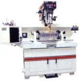
Rottler's SGF-8 seat and guide machine can handle a wide variety of cylinder heads from motorcycle heads to CAT 3406E heads. It features a fixed carbide pilot centering system, air float workhead with foot pedal control for hands free air clamping and digital electronic level for quick, precise alignment of fixed pilots.
