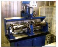
T&S Machines and Tools' XL2000 model seat and guide machine offers 2"more height and 10"more length for high performance work. This allows users to cut two heads in the same setup and all seats to the same exact depth.
