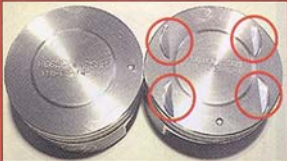
Figure 7 Early and late pistons are identical except for the four valve reliefs that were introduced in 2003 when the VVT engines came online.
