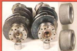
Figure 5 Crank forging number V 10 on left has shallow rear pilot hole with a depth of .524" and a bushing height of .970" (top view). Crank V1 60 on the right has a deeper pilot hole depth of .647" and a bushing height of 1.167" (lower view) which yield a protrusion height of .446" and .520" respectively.
