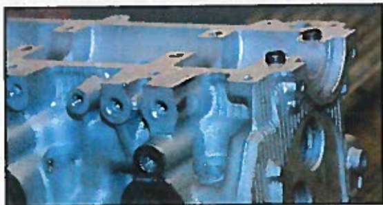
On the Toyota 3VZ, dowel pins locate the cam bearing caps at #1 and #5.
