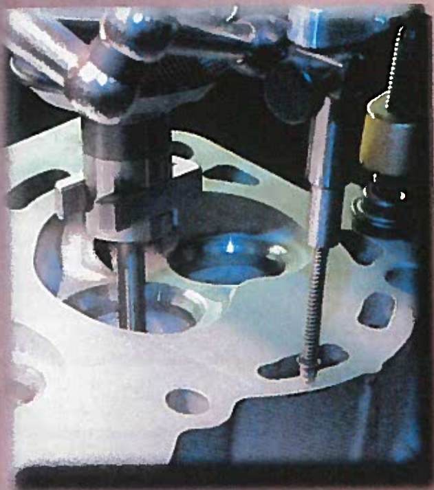
Finishing the valve seats on a Toyota 3VZ head with a Serdi 5.0. VEGE only allows .020" off seats before replacing.
