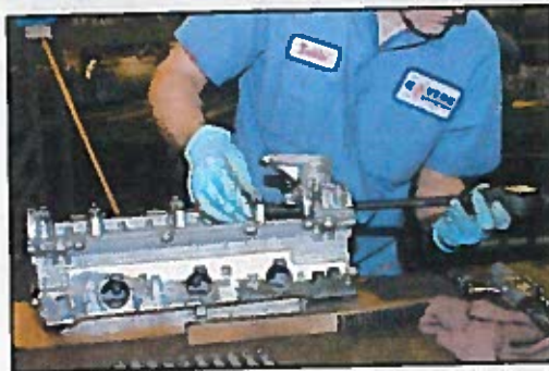
Checking the cam housing size after cutting and reinstalling the caps to determine if there is enough material to hone or bore to finished size. Caps can be re-cut if there is not enough clearance.
