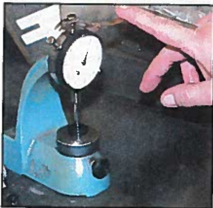
Checking a shim for proper size.
