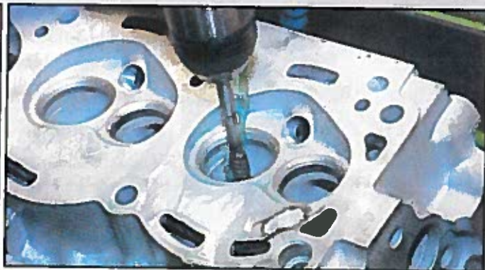
Diamond honing valve guide on a Toyota 3VZ head to remove nicks & burrs. Removes about .001"-.010".
