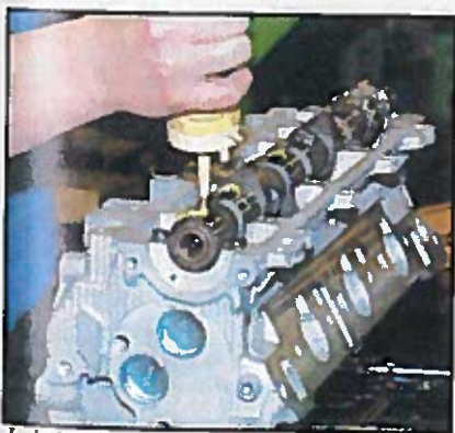
Lubrication is very important when reassembling an engine or head. When a newly remanufactured engine is first started it will run dry for several seconds and can cause damage if not properly lubricated during assembly.
