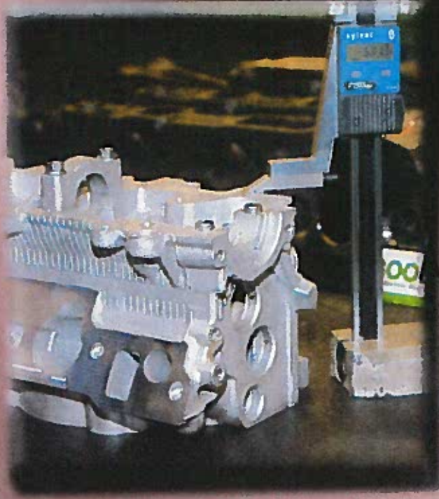
Checking the thickness of the head. You need to try to maintain OE specs to maintain compression ratio. With ORD II coming, maintaining OE specs will be critical.
