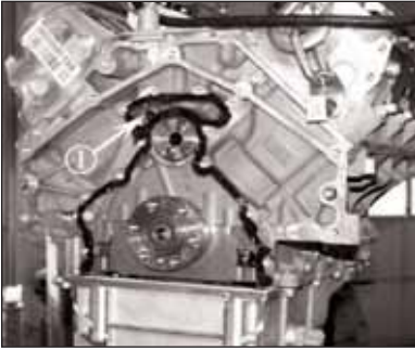
Figure 6 Rear engine oil leak on Isuzu Ascenders 5.3L engines.
