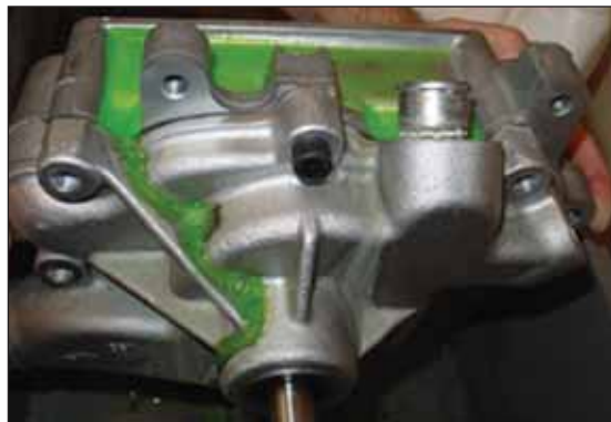
Figure 7 Coolant rolls across the front of the pump and behind the pulley, making it appear to leak from the weep hole.
