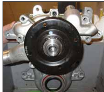
Figure 8 The pulley completely covers the face of the pump, making the correct diagnosis difficult.
