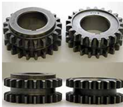
Figure 5 A shorter gear set was used prior to 2001/'02 and a longer gear after those dates.
