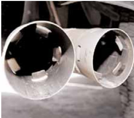
Figure 7 These exhaust tips should not be removed or covered with dress sleeves that will seal off the ports on the sides.
