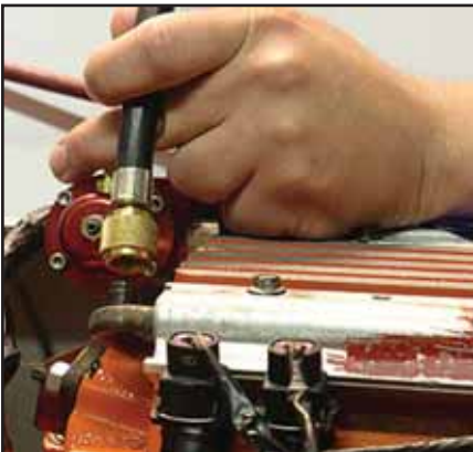
Figure 1 Screw the fuel pressure gauge onto the Schrader Valve located on the fuel rail.
