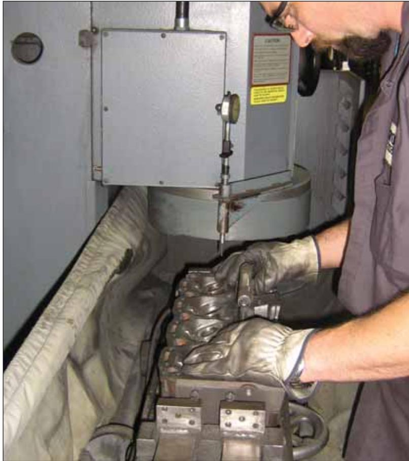
*Many late model engines are equipped with MLS head gaskets which help reduce cylinder bore distortion and typically have much lower clamping loads than traditional head gaskets. But they also require an extremely smooth, flat surface finish on both the block and head to seal properly, typically 20 to 30 microinches Ra (roughness average) or less.*
