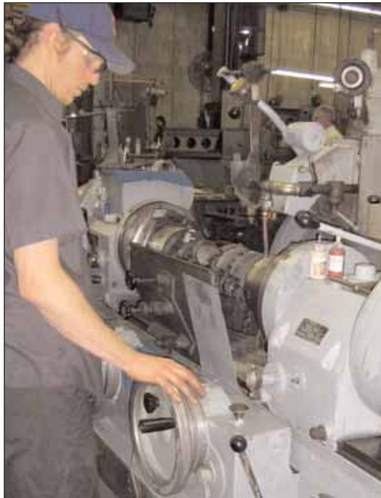
The amount of grinding that can be done on the crankshaft journals is limited by the depth of the case hardening as well as the availability of undersize bearings for the application (Photo by Doug Kaufman).
