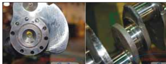
Figure 8 All IDI and IDIT engines in both 6.9L and 7.3L sizes use the same crankshaft (c/n 1085420C1).
