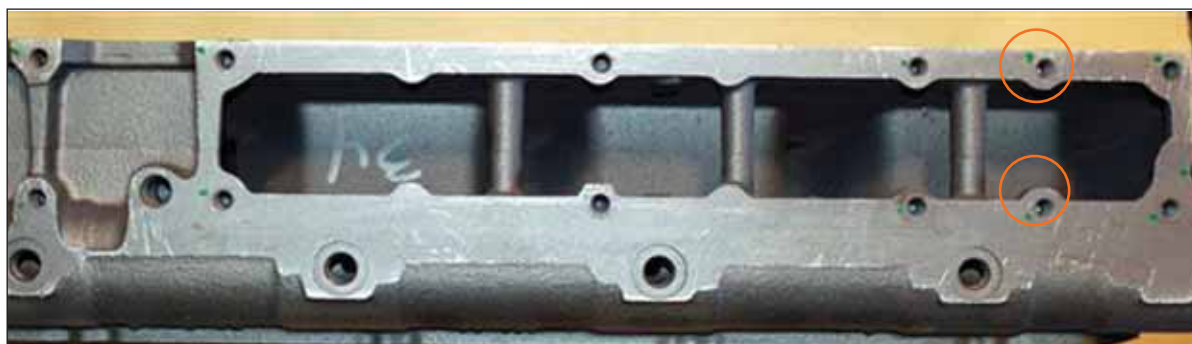
Figure 17 This is the 10-bolt intake manifold cylinder head from the 7.3L (s/n 896,813 to end). Earlier 8-bolt cylinder heads did not have the two bolt bosses circled above.
