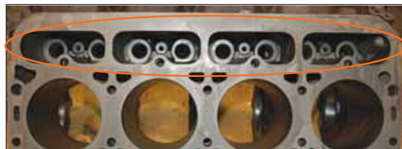
Figure 7 The second series 7.3L DIT block casting has solid casting support areas between each cylinder bore as well as additional crank counterweight clearance in the lower block.
