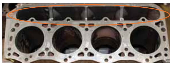
Figure 6 First series 7.3L DIT blocks had a large opening at the upper valley area of the cylinder head deck.
