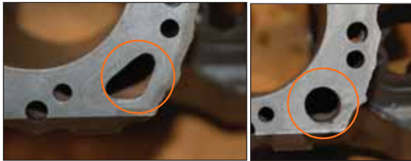
Figure 3 and Figure 4 The coolant port on the corner of the cylinder head deck is triangular on the 6.9L engine (left). The coolant port on the corner of the cylinder head deck is circular on the 7.3L engine (right).
