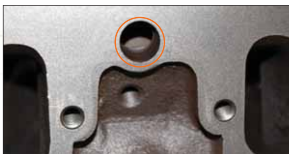
Figure 15 One of the second design 6.9L IDI head castings has the as-cast numbers ground off and the new one stamped in.
