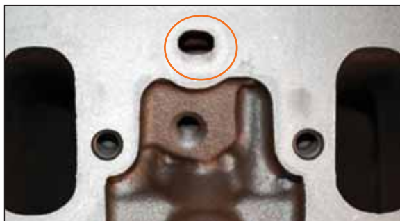
Figure 16 7.3L IDI and IDIT cylinder head castings may have two different shaped coolant ports. One is circular and uses a soft plug (top) and one is oblong without a plug (bottom). Both get covered by the gasket and both have c/n 1809030C3. They are fully interchangeable.
