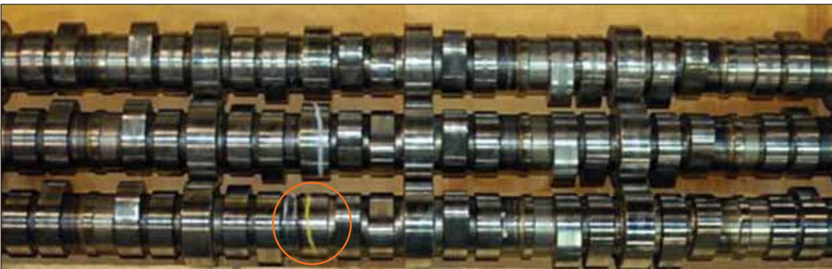
Figure 11 Three camshafts were used in the 7.3L DIT engine application. The top two cams are the standard duty camshafts, while the bottom one is for heavy duty Ford and Internationals from s/n 661,0974-2,030,402. Note the absence of the pump lobe.
