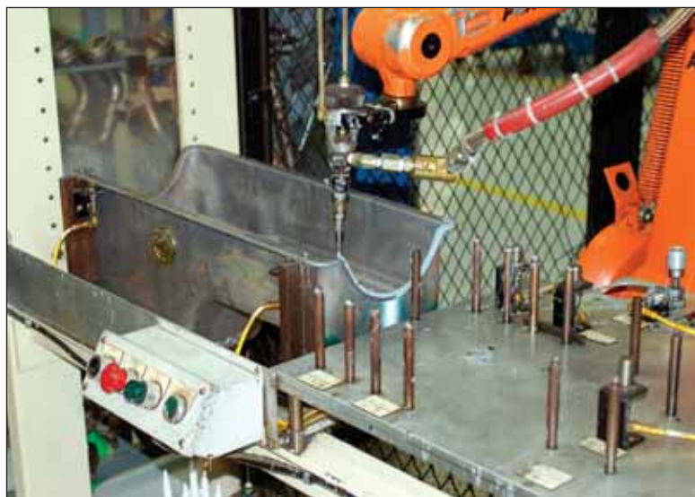
Figure 22 When it needs to be sealed right every time, a robot is used to apply the exact amount of sealer.
