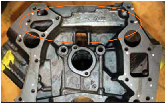
Figure 2 The second design 6.9L casting has a wide gusset across the top front of the block. This casting is considered the only viable casting for rebuilding by most.
