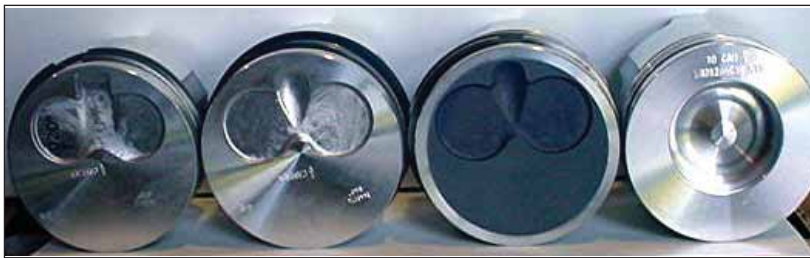
Figure 18 At right (reading left to right) a comparison of the four different pistons used from the start of production to the end of production. From left: 6.9L, IDI non-turbo; 7.3L IDI non-turbo; 7.3L IDIT; and 7.3 DIT turbo.
