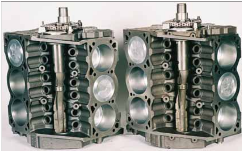
The only difference between the early and late Series II/III engines is the way the end seals for the intake are held in place. The early ones (left) slip over the rails while the late ones (right) are held in place with two pegs that fit into the blind holes on the outside of both end rails.
