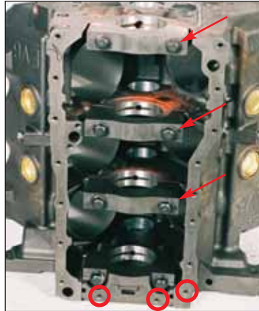
The '95 VIN L block was unique. It had powdered metal main caps and it used the '95 VIN K bolt pattern for the pan gasket, so three of the bolt holes (circled) were moved.
