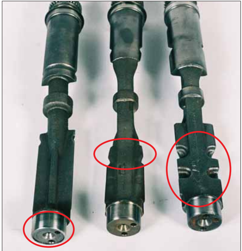
The 24502389 balance shaft on the top was used for all the FWD applications from '88-'95. The 334 that had two notches in each counterweight, (middle) was used in the regular Series II/III motors and the 336 that had four notches in each counterweight was used in the Series II/III supercharged motors. Notice the wear sleeve on the early one, too.
