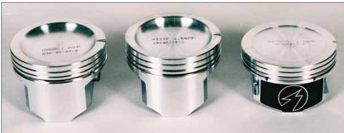
The naturally aspirated motors used three different pistons since '88. The '88-'92 is on the left, the '93-'95 is in the middle and the '95-'08 VIN K/2 is on the right.
