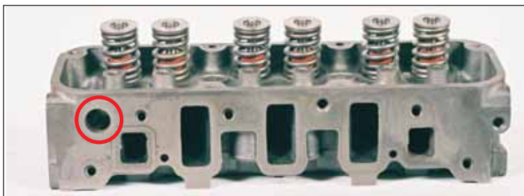
The head used on the '90-'92 VIN L motors had seven bolt holes for the intake and a large vent hole in the intake surface.
