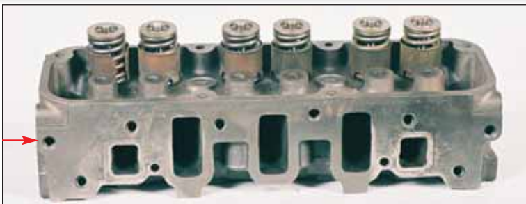
The head for the '88 VIN C had eight bolt holes plus two blind holes for the dowels that were used for the intake gasket. The upper left hole wasn't drilled when it was used on the '89-'91 VIN C.
