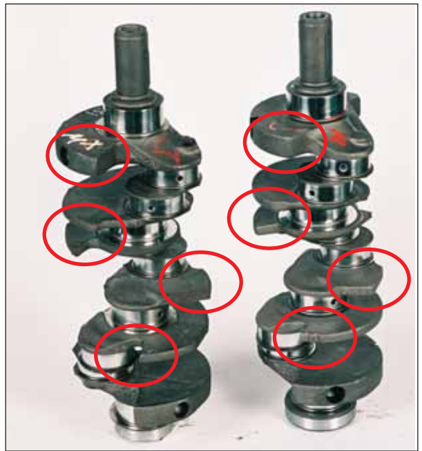
There's a lot of difference between the original FWD crank (left) and the lightweight version that was used in the Series II/III motors. The counterweights tell the story.
