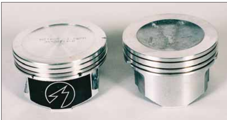
The piston for the Series II supercharged engine (right) is quite a bit different than the one that was used in the naturally aspirated engine.
