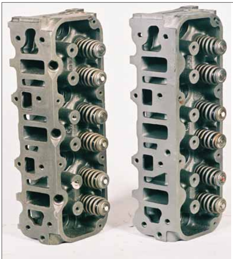
The heads for the supercharged Series II/III engine have three holes above the intake ports for the injectors because there wasn't enough room for them in the intake manifold when the supercharger was installed.
