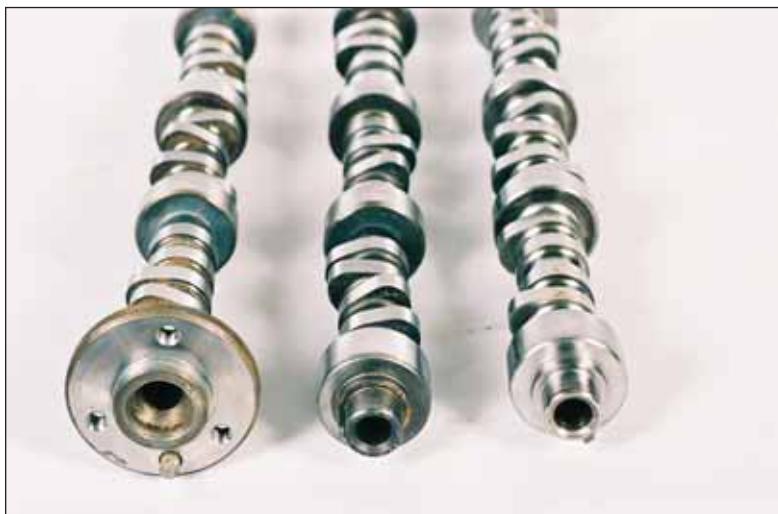
The cams that were used from '88 and up are noticeably different. The flanged version ('88-'90) on the left was replaced by the one with the threaded hole instead of a flange (middle) that was used from '91-'95. The Series II/III cam on the right ('95-'08) still had the threaded hole, but it had bigger journals (1.845" vs. 1.785").
