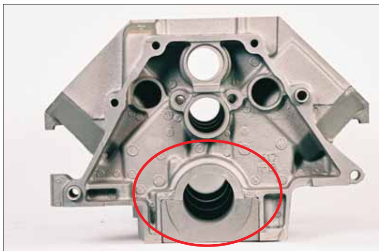
The '88-'90 VIN C engines still had a two-piece rear seal.
