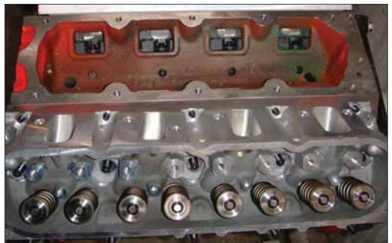
The L92 cylinder heads have a performance lineage, even though they're seen predominantly on trucks and SUV's. For our application, they were the perfect addition, once we CNC ported both ports and decked the heads slightly.
